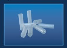
Mylar is the most recognised and industry approved sleeve material. Industrial Gaskets recommends Mylar Sleeve as it is stronger than Phenolic and less prone to cracking during the installation process. It is available in both Metric and Imperial sizes. The standard length is 900mm or 3Ft and can be supplied in full lengths or cut to suit your bolt length.
