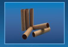
Phenolic has been a cheaper alternative to Mylar in years of the past. However, it is prone to cracking or splitting during the installation process as the material can be brittle, especially under high bolt torque. It is available in both Metric and Imperial sizes. The standard length is 900mm and can be supplied in full lengths or cut to suit your bolt length.
