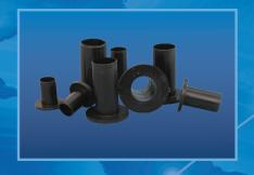
Tough, convenient-to-use, cost effective, one-piece sleeves and washers are available moulded from Mineral reinforced Nylon-Minlon®. TopHats reduce handling and make-up problems in the field. They are moulded to specific lengths and are in many instances longer than the thickness of a single flange. Minlon® has an excellent dielectric strength and high compression strength. Industrial Gaskets Top Hats also contain a UV stabilizer.
