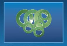
G10 / G11 Glass Epoxy washers are tough and recommended where high bolt torque is required. Glass Epoxy maintains good dielectric and physical strength where some other materials weaken. Standard thickness is 3.2mm. Other thicknesses available on request. G10/11 has a dielectric strength of 530 VM, Water Absorption of 0.09% and maximum continuous operating temperature of 140°C.
