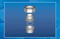
Ground Joint connections provide a long reliable life with a seal that is widely used in the oil and gas industry. "O" Ring Unions provide a leak proof static seal. They can be used and removed in the field without replacement or damage to the insulator. Their dielectric strength goes beyond the toughest requirements. Ranging up to 3000psi and sizes 1/4" up to 3".
