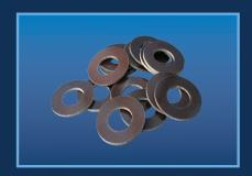
Standard insulating washers are made of high strength phenolic and provide positive insulation at temperatures to 120oC. They are made to fit over the insulating sleeves. Standard thickness is 3.2mm. Other thicknesses available on request. Phenolic washers are not recommended where high bolt torque is required as they tend to crack. Phenolic has a dielectric strength of 400-500VM with a water absorption rate of 1.1%.
