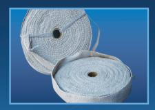
Ceramic Fibre Tape is manufactured from ceramic fibre yarn which is reinforced with either glass or inconel wire. It is suited for high temperature, low pressure applications where poor flanges or low bolt loadings are present. Typical applications are for ductwork flange gasket, furnace / boiler door seals and cable and pipe protection. Ceramic Tape is rated to 1000°C.
