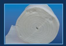
The Ceramic Fibre Blanket has excellent thermal stability and thermal shock resistance. This material has low thermal conductivity, low heat and storage. Temperature rated to 1260°C. Applications including furnace lining of every type, industrial furnace and heating equipment, metallurgy, machine construction and materials, petrol and chemical engineering.
