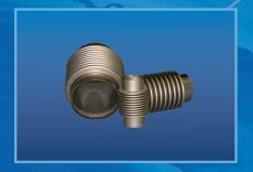
Metal Expansion joints or Exhaust Bellows are the most important part of an exhaust system as they act as a shock absorber isolating engine vibration from exhaust systems to avoid metal fatigue and ultimate failure. The bellow is made up of a series of convolutions which assist in the axial and lateral movements.
