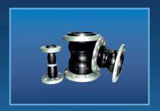
Twin Sphere Rubber Expansion joints are ideal for applications requiring large axial, lateral and angular movements. They contain floating flanges (non fixed) to allow for easy alignment in a range of materials including 316 Stainless Steel, Mild Steel and Galv Coated.
