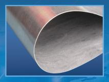
GraphTek 5130 is a compressed proprietary fibre sheet, combining a high percentage of graphite, reinforced with aramid fibres and a NBR binder. An excellent gasket sheet for high temperature and pressure. It is produced under high load which ensures the material has very low gas leakage. Because of low tensile strength and low gas tightness, GraphTek5130 is much more restricted in application.
