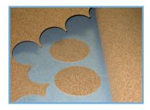
Cork Sheet material is manufactured with NBR binders. One of the main applications is transformers in the power service. It has a high compressibility and moderate resistance to most oils. Ideal where light bolt loads only are available and pressures are low. Pressed steel flanges and uneven surfaces are easily sealed due to the high deformation of the cork. Operating temperature of 120°C.
