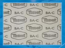
TESNIT® BA-C is specially developed soft gasket material for the chemical industry. It is a sealing material based on aramid fibres and CSM rubber. The material has very good resistance to acids and alkaline media. It is also very convenient for the different aggressive media. TESNIT® BA-C finds the application in all places where the chemical resistance is the most demanding factor. Gasket material with very good resistance to acids and alkaline media.
