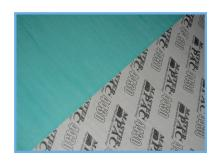
MP4430 is a compressed proprietary fibre sheet, combining aramid fibres and a NBR binder. A good and reliable general purpose, high temperature and pressure sheet. Has superior sealability with excellent oil resistance. Water treatment plants, chilled and cold water lines / hot water and service steam, oil, fuel and alcohols / compressed air, gases (incl. oxygen), moderate organic & inorganic acids.
