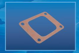
Doniflon 2020 is biaxially orientated PTFE sheet produced from virgin PTFE resin filled with silica. This material is particularly suitable for use with strong acids, except hydrofluoric acid.
