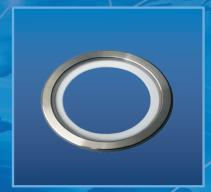
Ring Type Joints can also be supplied with PTFE inserts, in order to reduce turbulent flow and eliminate gasket/flange erosion. The insert is specially designed with radially drilled pressure passage holes so that the self energising performance of the Ring Joint is not impaired.
