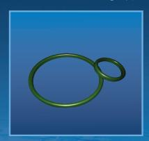
This is a Ring Type Joint totally enclosed in a PTFE coating. The RTJ material is usually soft iron or low carbon steel. This type of gasket is predominately used in aggressive media applications. Coating can be in various colours eg blue or green for ease of identification on site.
