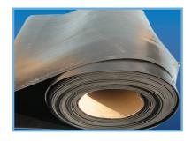
Butyl Rubber is a fully synthetic rubber made from 100% Bromo Butyl Polymer. Butyl Rubber has excellent chemical and heat resistance with low permeability to air and good weathering properties. It has however poor resistance to petroleum based fluids. It has high resistance to permeation.
