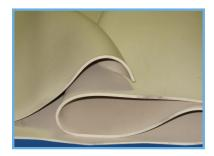
A high grade natural rubber with good all round properties, including resistance to abrasion. Available with no insertion or 1 ply or 2 ply insertions. Meets with requirements of FDA Part 177, making it suitable for use in food manufacturing and handling applications. Can also be used in flange isolation.
