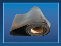
A fully synthetic rubber made from 100% EPDM Polymer. It also has basic resistance to some chemicals and acids. EPDM rubber has good ozone, weathering and temperature resistance. It is used for sealing against diluted and highly concentrated acids and lyes. Available in Potable Water Certified to AS/NZS4020 drinking water standards.
