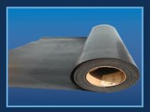
Natural Rubber has good all round properties including resistance to abrasion. It has relatively low resistance to temperature and petroleum based fluids. It has excellent mechanical properties, good ozone, acid and alkali resistance, but not adequate for use with oils and solvents. It is available with 1Ply or 2 Ply cotton or nylon insertions for reinforcement.
